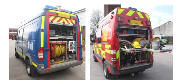
**11.13** Both services with the Mercedes type vehicle were In agreement that the overall stowage and type of the equipment carried was good Based upon incident need and type, this being the second generation TRV so it has been tried and tested with the specification already in place. NFRS will identify the equipment to be carried by referring to current suppliers and need.
